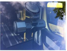
introduced CCTV alongside our tracking and scheduling technology. All new dial-a-ride vehicles now have on-board CCTV. The CCTV records the road ahead and also an image inside the vehicle. Data is held on the device for a couple of days and then overwritten. Should an
