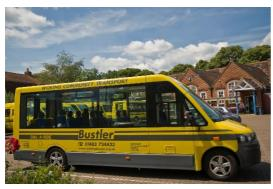
include low-floor variants which have proved popular with some of our wheelchair users. The low-floor vehicle allows us to transport electric wheelchair users without the need for a passenger lift, thus reducing risk when entering and exiting the vehicle.
